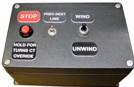
Button Box for most operations while winding
