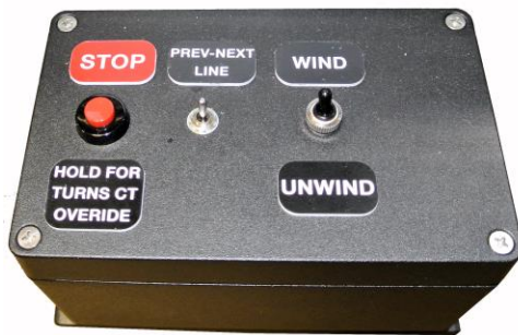
Button Box for most operations while winding
