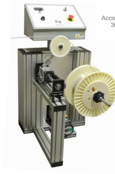
OTT-Mini Accommodates spools up to 20 inches in diameter weighing 40 pounds
