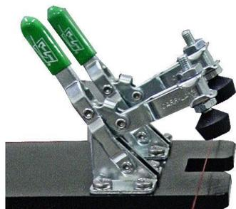
**Wire Clamps** – A pair of manually operated clamps are positioned in the path of the wire. While spooling, the clamps do not interfere with the motion of the wire. They can be lowered before a cut is made and provide a repeatable cutting location. They also allow the operator to maintain control of both ends of the wire so that the coil can be processed and the new end quickly secured to the take-up for the next spool or coil to be made.
