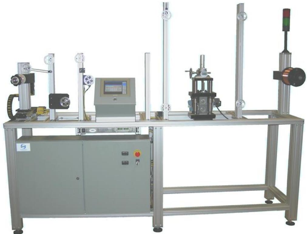
CE version of wire flattening mill includes interlocked safety guards
