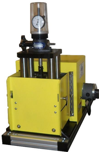
CE version of wire flattening mill includes interlocked safety guards
