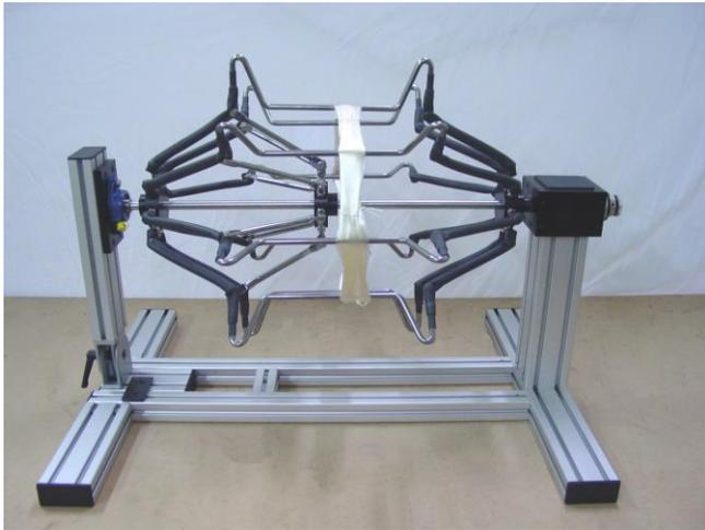
Payoff unit for Hanks and Skeins. The linkage adjusts to accommodate different diameter loops.
