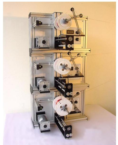
Modular Take-up System (MTS) with Closed-Loop Tension Control
