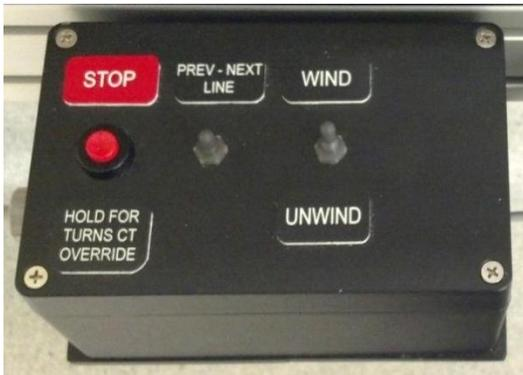
*Button Box for most operations while winding*
