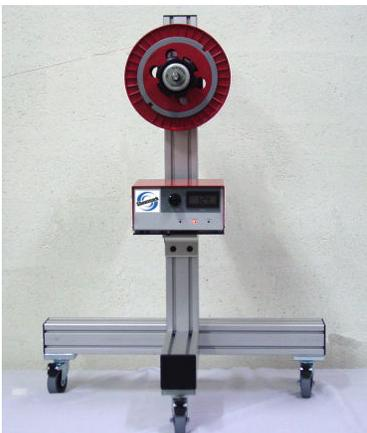
Basic Payoff with Closed-Loop Tension Control
