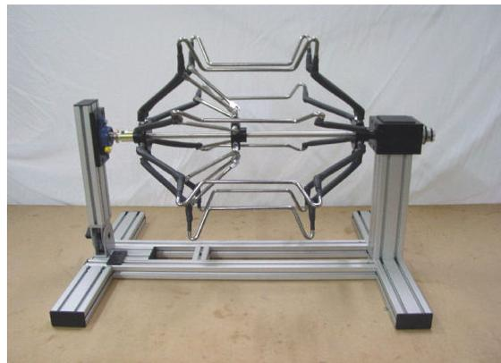
Payoff unit for fishing line skeins and textile hanks. The linkage adjusts to accommodate different diameter loops.
